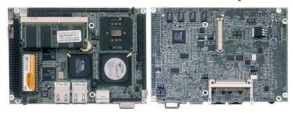
The HS-2608 v2.0 is a VIA VT8606 chipset-based board designed for Mini PCI Local Bus and use ULV Intel® Celeron® processor 400MHz/650MHz. These features combine and make the HS-2608 v2.0 an ideal all-in-one industrial single board computer. Additional features include an enhanced I/O with CF, CRT/LVDS, dual LAN, audio, 4 COM, and USB ports interfaces.
